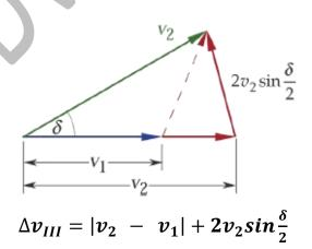
**NOTE:** Since the sum of the lengths of any two sides of a triangle must be greater than the length of the third side, it is evident from above figures that both  $\Delta v_{II}$  and  $\Delta v_{III}$  are greater than $\Delta v_I$ . It follows that plane change accompanied by speed change is the most efficient of the above three maneuvers.
